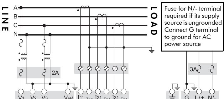
Phase B voltage ( $V_2$ ) is derived from phase A and C voltages.
