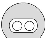
The infrared serial communications port can be used for energy pulsing or communication with Schneider Electric power monitoring software.
