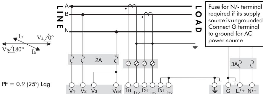
For this configuration ONLY, the 208 V line-to-line voltage inputs can be used with 240 V line-to-line systems.
