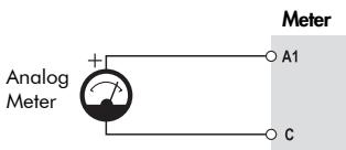
Example application: driving an analog meter with the DC current output.
