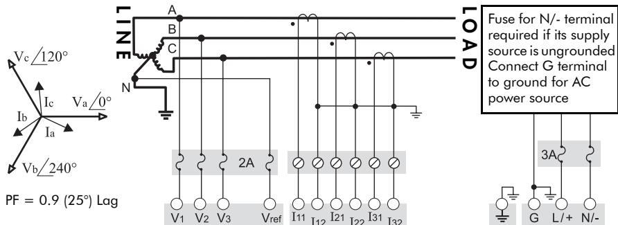
The configuration requires that the transformer secondary star-point is grounded. The phase-to-ground voltages must be within the meter's range.
